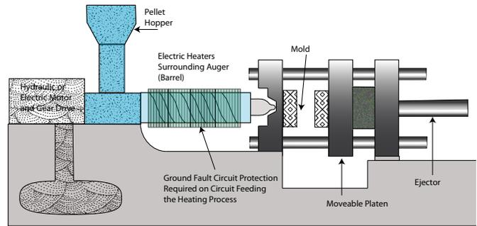
In a plastic injecting molder application, the plastic pellets are melted using electric heater bands between the hopper and the nozzle directing the plastic into the mold. If the heaters fail, the best approach is to let the process complete rather than disassembling the machine to clean out the solidified plastic.
